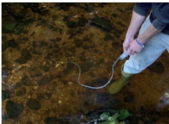
Syringe for sampling interstitial water.
